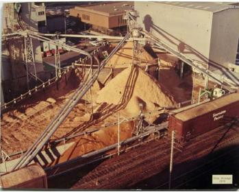
Here you can see a pile of wood chips in 1979 on their way to being cooked and ground into pulp at the paper mill.
